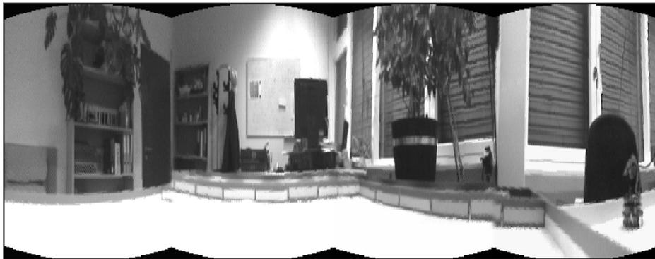
**Figure 5.2:** A view taken by the Khepera in the “Office” environment. Four camera images are merged into one panoramic view, covering about 240°.
